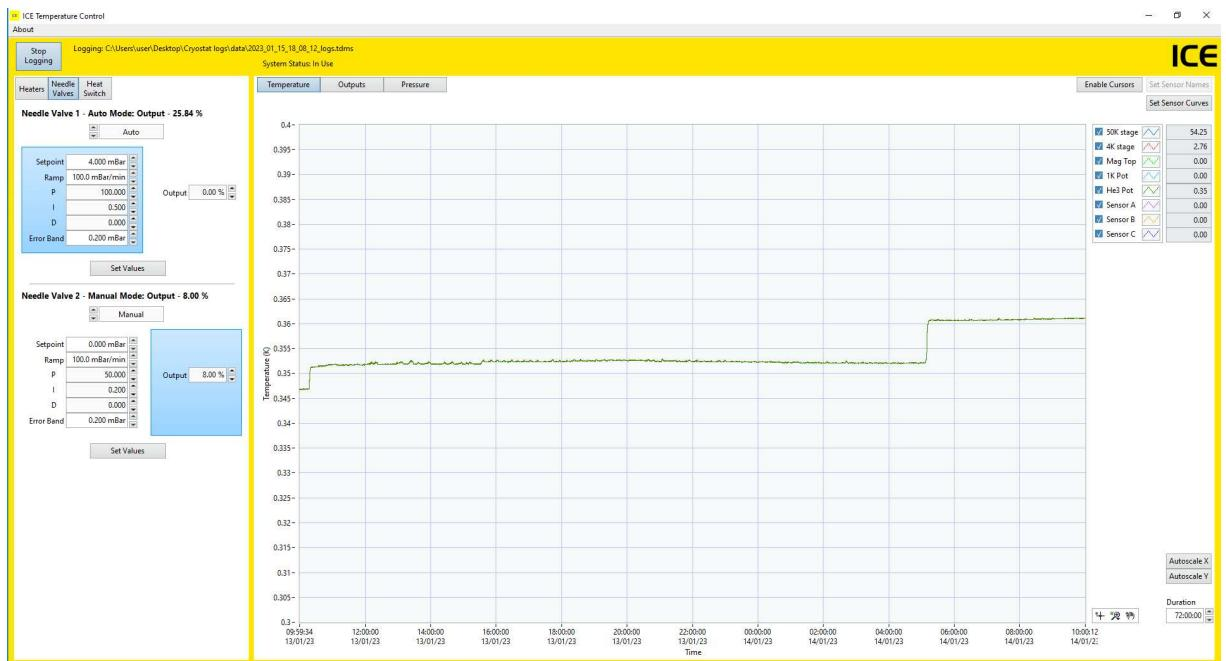
100  $\mu\text{W}$  cooling power (0.89% on Heater2): T=352 (jump to 360mK at some point) (NV2=10%; P1,3=293mbar)
