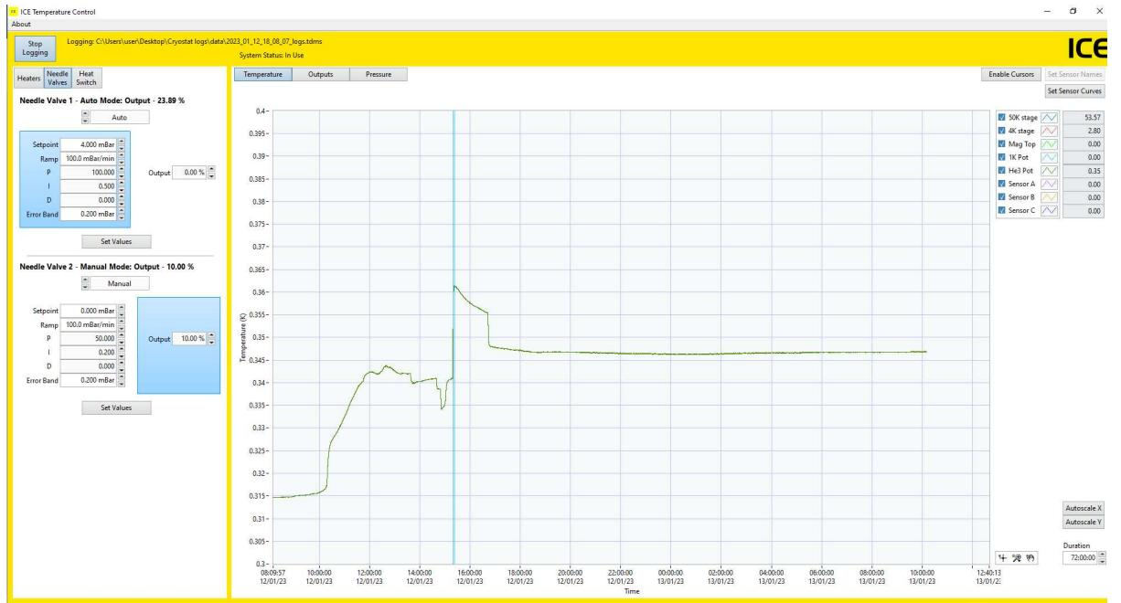
50  $\mu\text{W}$  cooling power (0.6% on Heater2): T=347mK (NV2=10%; P1,3=260mbar)
