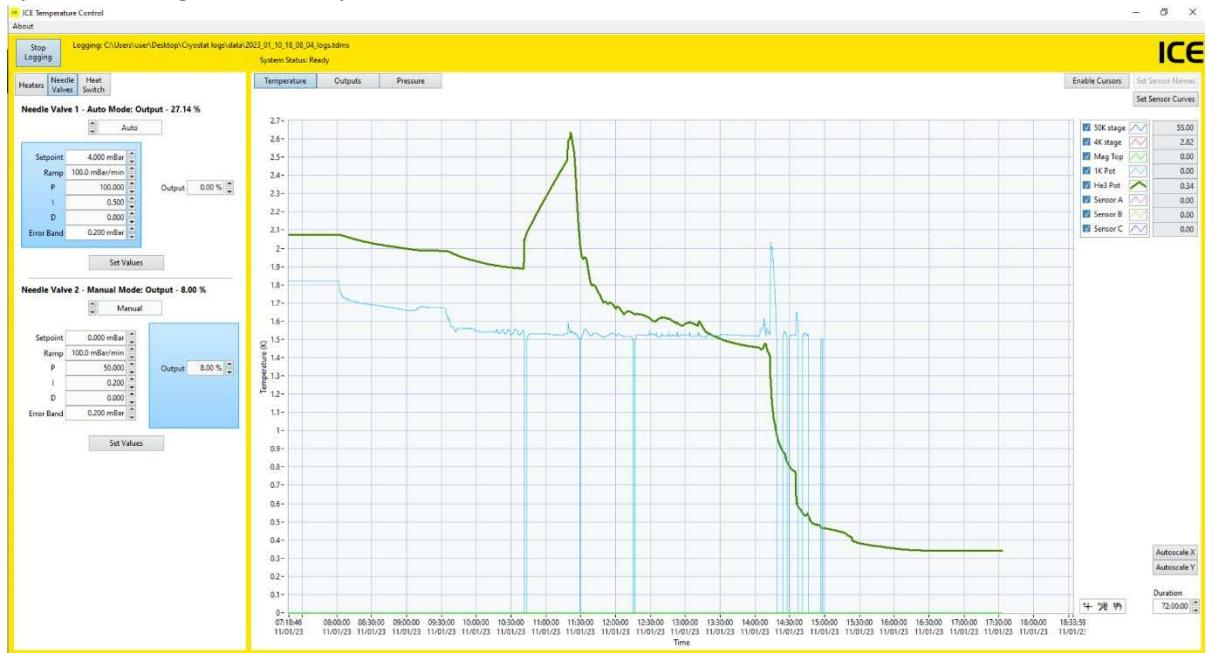
After leaving overnight to stabilise system reached a continuous base temperature of 315mK. Base in continuous mode: T=310-315mK (NV1=4mbar, NV2=8%; P1,3=50mbar)
