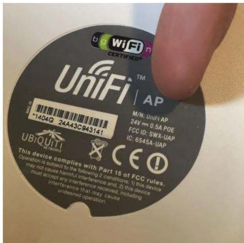
Figure 1. This AP requires a Passive PoE 24v supply. It can be confusing, because even though it says it's PoE, it won't power on using a standard 802.3af switch.
