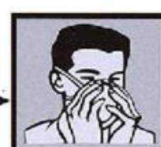
5. Test the fit. Cup both hands over the respirator and exhale vigorously. If air flows around your nose,tighten the nosepiece.
