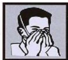
4. Using both hands, mould the nosepiece to the shape of your nose.
